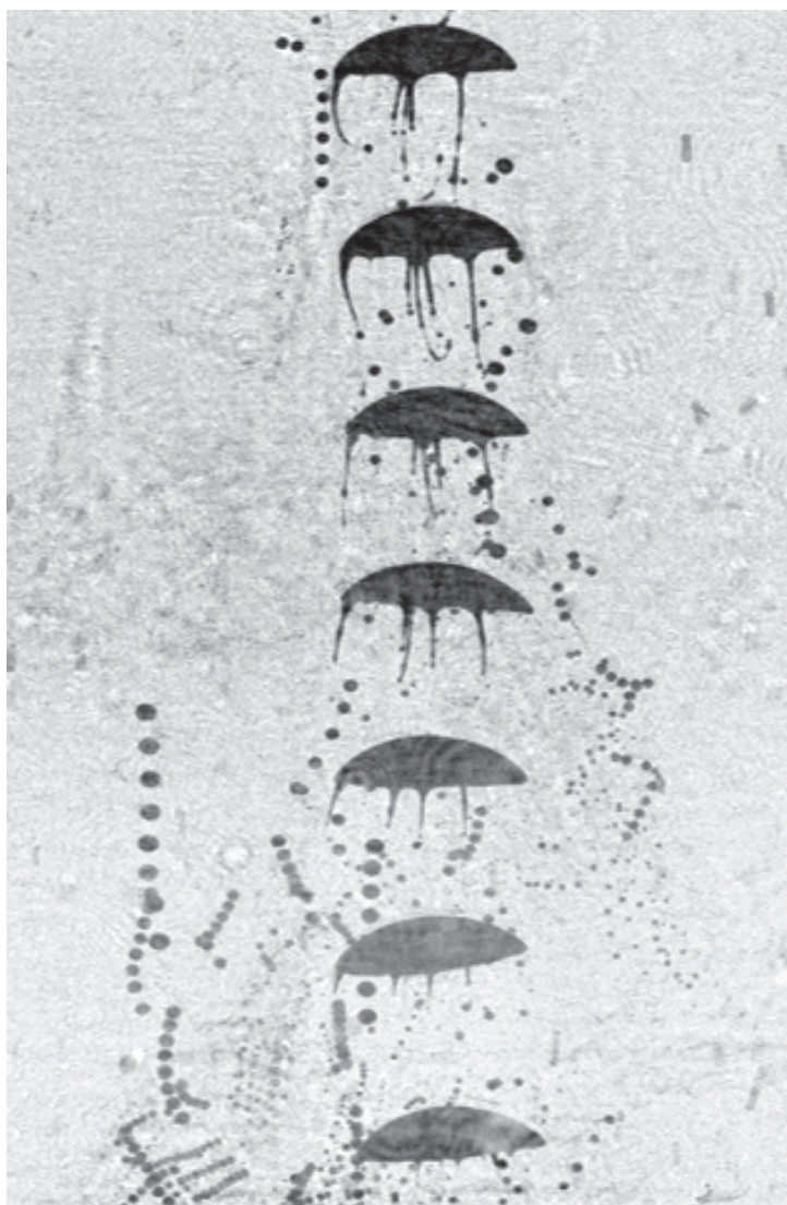
"Octopus" oil droplets are generated when oil premixed with dispersants is released in the water column. (Chang Li and David Murphy/DROPPS photo)
