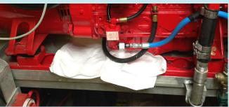
Oil absorbent booms, sheets (bottom), and pads can be kept on your boat to catch leaks under the engine or to contain and remove oil at the surface of the water (back). Bilge socks (top) trap any oily overflow on board, making safe disposal easy. (MASGC/Tara Skelton)
